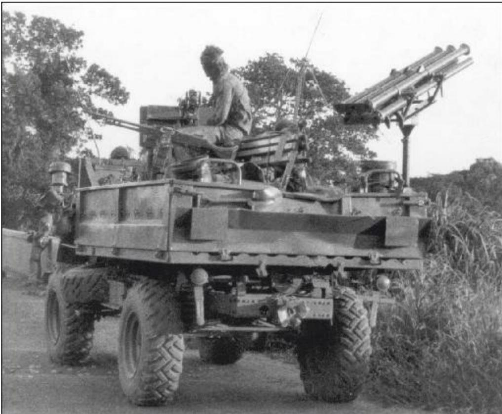
Unimog with home-made mounted SNEB (white phosphorus) and armour-piercing rocket launcher.
