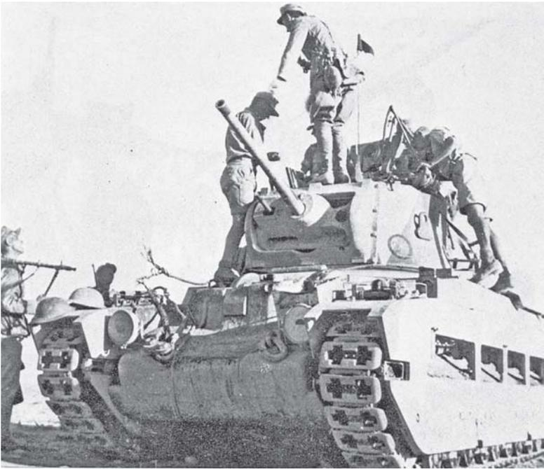
The heavily armored British Matilda Mark 2 infantry tank. Relatively impervious to the standard German antitank guns, only the famous "88" could knock it out at long range.
