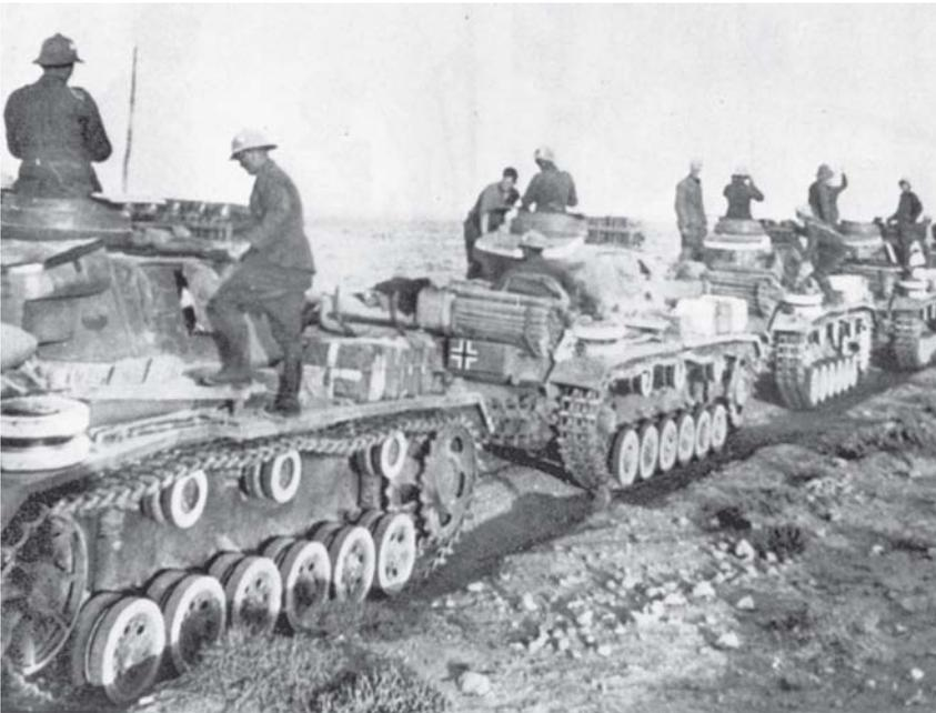
*Panzer III*s head for the front in the early stages of the campaign. Note the fuel and water (marked with a white cross) containers at the front of the tanks and the extra stowage of essential items.
