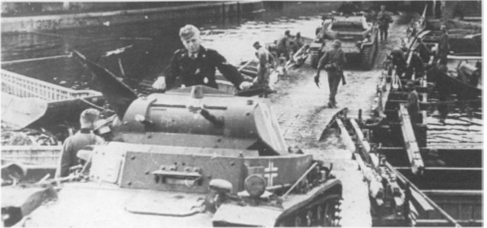
Above: PzKpfw IIs of Pz Regt 25 crossing a bridge built by 7 Pz Div's engineers across the Canal de la Bassée. Note the muzzle covers on the 20mm cannon and MG 34 (to keep the dust out). The tank commander wears the Iron Cross 2nd Class, plus a panzer assault badge. (Tank Museum)
