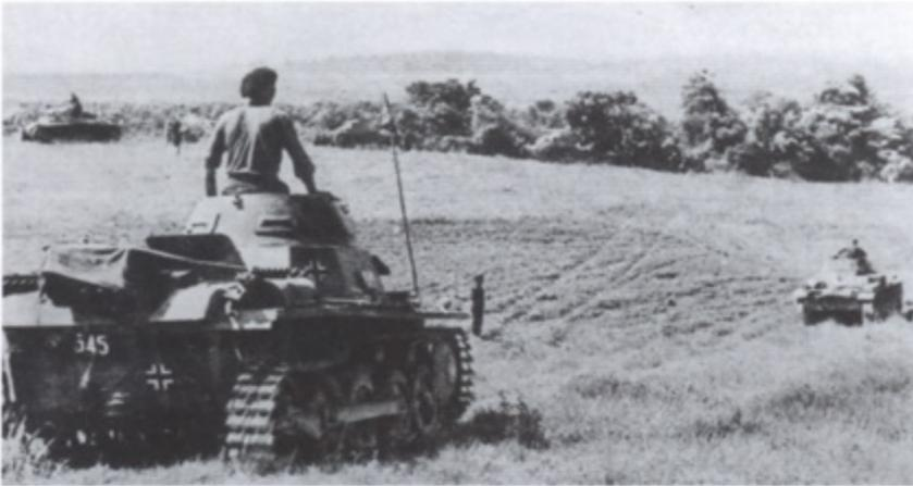
A Panzer regiment on field exercises, summer 1939. In the foreground is a Panzer I light tank, ahead of it a light Panzer II armed with a 20mm gun. To the left, in the background, are a Panzer III and Panzer IV medium tank, the first armed with a 37mm gun and the latter with a short-barrelled 75mm. (Private collection)
