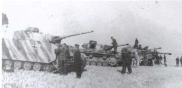
Though outdated, the Panzer III was still in widespread use throughout 1943, and the tank carried on in production till August of that year. This is a typical mixed unit on the Eastern Front equipped with both the Panzer III (one of them with a flamethrower) and the Panzer IV. (Nik Cornish, WH 821)
