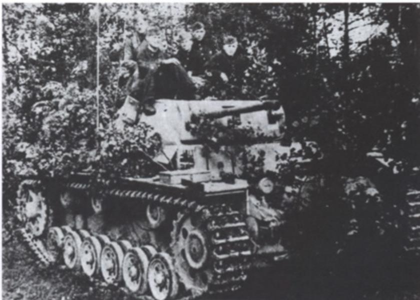
A camouflaged Artillerie Panzer Beobachtungswagen III, an armoured artillery observation vehicle based on the Panzer III tank developed in February 1943, in use by armoured self-propelled artillery units, an organic part of the Panzer divisions from that year. (Carlo Pecchi)
