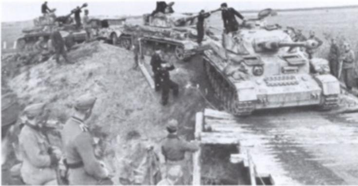
A column of late-model Panzer IV Ausf. G tanks crossing a Russian river over an improvised bridge, 1943–44. Although it was not the best tank in the German inventory, the production of the Panzer IV was continued on Guderian's advice in order to provide a suitable main battle tank until the Panther became available in large quantities. (Private collection)
