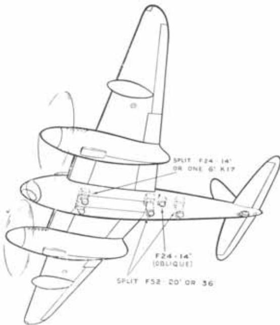
**Photo 5:** (above) Camera locations in the Mosquito. **Photo 6:** (right) A 36-inch (90-centimeter) camera in position that could obtain large scale images from high elevations.
