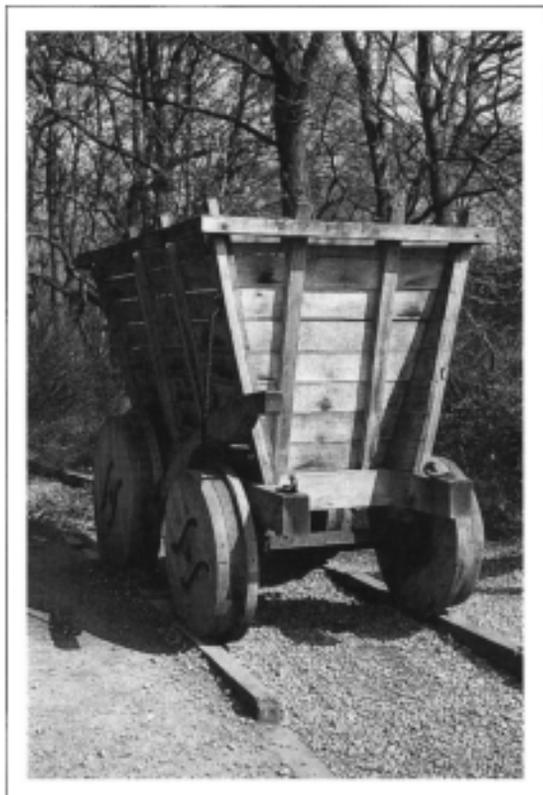
**Figure 16.7** Reconstruction of a coal wagon on a wooden wagon way, Causey, Durham.
