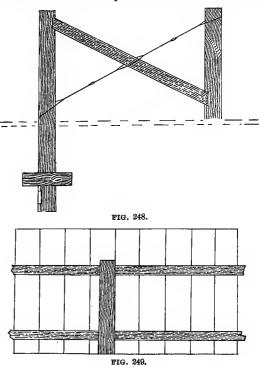
also, and a fence built on well-set posts and thoroughly nailed will never sag or get out of line until the posts rot off.
