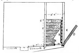
FIG. 324-WING'S COW STALL SHOWING CEMENT FLOOB.
