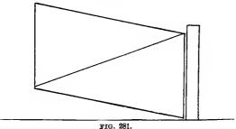
to position shown the gate should be in the same shape as Fig. 281. This gate must be bolted together, one bolt at each intersection.
