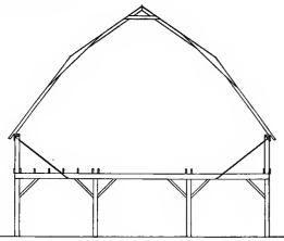
END ELEVATION OF FRAME FIG. 97-HORSE BARN WITHOUT CROSS-TIES
