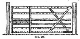
many or few horizontal bars. The drawing shows six bars which cut 1''x4'' and properly spaced make the gate just 5' high.
