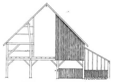
FIG. 174-SBEEP BARN WITH GLASS COVERED LAMB SHED (END ELEVATION).
