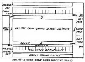
The plan indicates a barn  $50' \ge 70'$ , with cattle stalls and a 3' alley on each side, central space and entire area above the stalls being devoted to the mowing of hay and straw. The "end section" (Fig. 67) is intended to show this arrangement.
