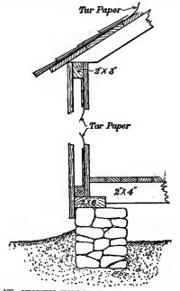
FIG. 189-SHOWING HOLLOW WALLS AND FOUNDATION.
