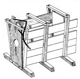
FIG. 301-A BACK FOR DEHORNING CATTLE AND FOR BINGING HOGS (SIDE AND FRONT VIEW).
