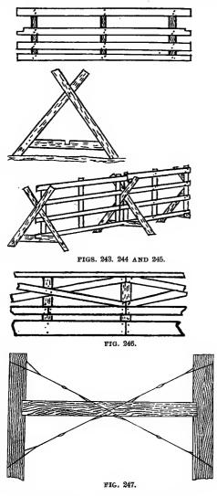
frame, as shown in Fig. 245, making a very strong fence. This is a very handy fence for fencing temporary pastures and is often used to divide a pasture from tilled land.
