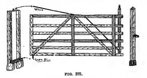
clear of the ground. A post to which to latch the gate when open will be found convenient, for when properly hung the gate will not stand open unless held.
