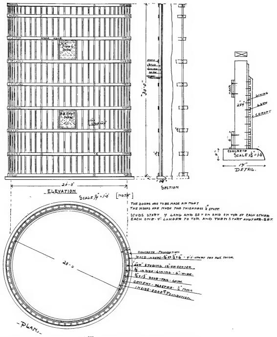
FIG. 207-CONSTRUCTION AND TYPE OF ILLINOIS SILO.
