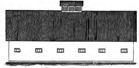
FIG. 68-A CORN-BELT BARN (SIDE ELEVATION).
