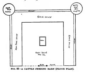
Two silos are provided having a capacity of more than 200 tons each. The doors for emptying are inside the sheds and there may be an overhead track carrying a large box along the line of
