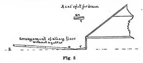
instead of the gutter a drop be arranged, as shown in Fig. 5. T and U are made of a  $2'' \ge 6''$ , split diagonally.
