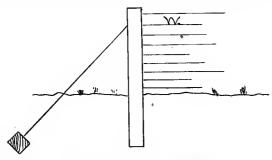
FIG. 258-BRACING A WIRE FENCE.
