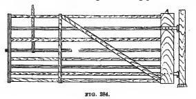
bottom hinge must be put on the side where the gate is to open. Make the gate, put on the hinges and then plumb it. Mark where to bore holes in the post while the gate is standing propped up against the post. Any one can make and hang such a gate.
