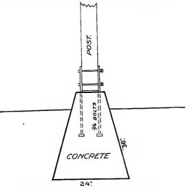
FIG. 297-ANCHORING A BARN TO THE GROUND.
