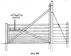
a sliding 4" stick with notches cut in it so as to keep the latch in place when open or closed.
