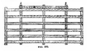
half the upright pieces in place. It will be noted that the braces A B are bolted through the rail next the bottom at C, and the other bolts merely pass through the braces either above or below the rails, as shown in the drawing. The connecting pieces D must be just  $\frac{2}{3}$ " above the
