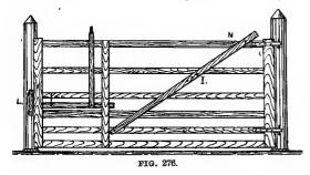
gate. At L two strong pins are put in the post with a  $1\frac{1}{2}$ " or 2" auger, with a 1"x8"x15" board nailed on as shown, with the side next to the gate dressed. The inner edge of the board is about 1" from the gate and just far enough from the post for the latch to pass behind it freely; the outer edge of the board should be at such an angle from the gate as will cause the latch to strike it near the outer edge; this causes the latch to swing back and glide in easily.
