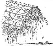
FIG. 306-DEVICE FOR COVERING STACKS.
