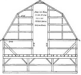
FIG. 2-WING'S JOIST FRAME.
