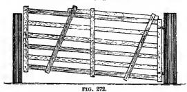
ward the end of the gate drops to the ground and this serves to keep it open when desired. The hinges are common strap and screw hinges, the strap bent around as shown in Fig. 272 and bolted to the vertical pieces:
