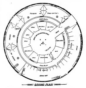
FIG. 13-NEW TYPE OF CIRCULAR BARN (GROUND PLAN).
