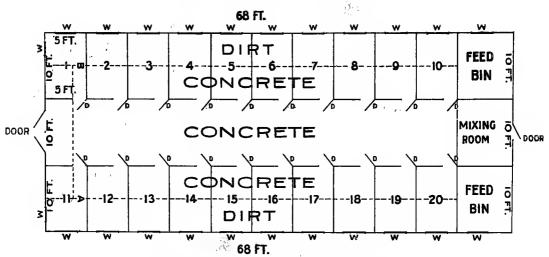
FIG. 149 HOG HOUSE FOR SOWS AND PIGS (GROUND PLAN).
