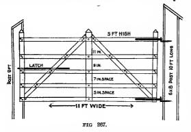
The latch is placed in the gate between the brace boards, which are double, one on each side of gate, as also are the end and center pieces. Use two bolts in each board as shown in the cut. It holds the gate in place better than when one bolt is used. Forty-eight  $3\frac{1}{2}"x\$"$  bolts are required. The cost is about \$6 for painting, building and lumber.
