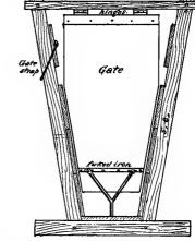
FIG. 300-A RACK FOR DEHORNING CATTLE AND FOR RINGING HOGS (END VIEW).
