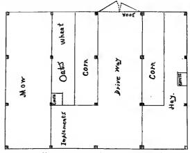
FIG. 29-A BANK BARN (FIRST FLOOR PLAN).
