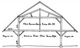
FIG. 213-TOOL HOUSE AND WORKSHOP (CONSTRUCTION).
