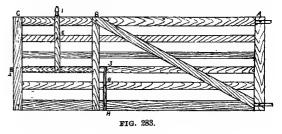
the gate from on horseback. 1, of course, is the latch handle working on a bolt at E; 2 is the latch proper; 3 is the latch spring fastened at H and G with the upper end bolted to the end of the latch.
