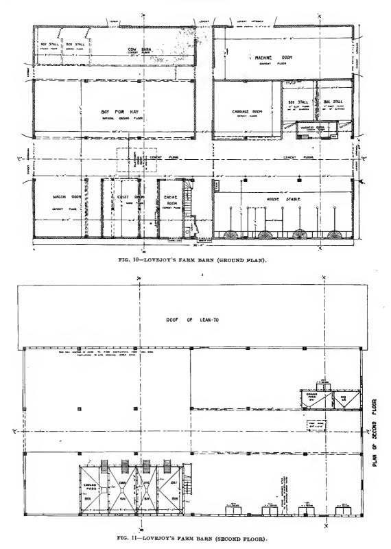
on the cement, as it was thought that horses would be less liable to slip. A drilled well is in the stable with a 100-barrel tank above in the second story. A system of water works from the elevated tank in the barn furnishes a good supply of water in the barn and out in the yards.
