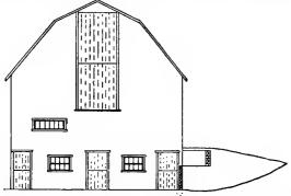
FIG. 110-BANK STABLE FOR HORSES' (FRONT ELEVATION).
