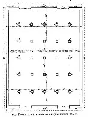
oughly in these barrels and when it became hard the hoops on the barrels were cut and the staves removed, leaving a round concrete pier on which to lay the stone caps.
