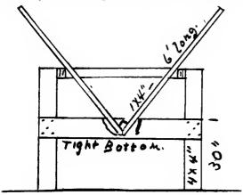
FIG. 235-COMBINED HAY AND GRAIN RACK.
