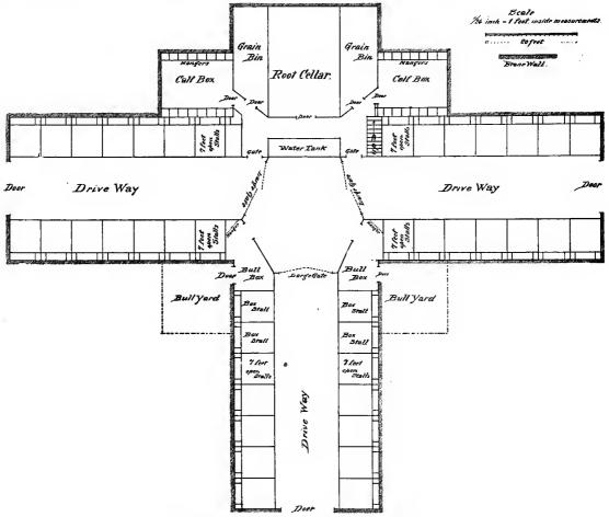
FIG. 18-A STOCK AND HAY BARN (BASEMENT PLAN).
