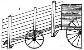
FIG. 307-A PORTABLE HOG-LOADER.
