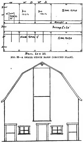
FIG. 36-A SMALL STOCK BARN (END ELEVATION).
