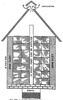
FIG. 308-A FARM ICEHOUSE (CROSS SECTION).
