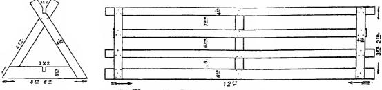
FIG. 253-PORTABLE HOG AND SHEEP FENCING.
