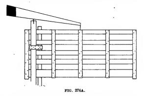
what the heft of the gate is when finished the lever can be weighted until a small child can open or shut the gate with ease. This gate swings only one way.
