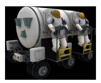
NASA has even generously provided an image of a proposed lunar rover with two integrated suitports, as seen above. The agency feels that such technology will be required for any 'return' trips to the Moon or for landing on
