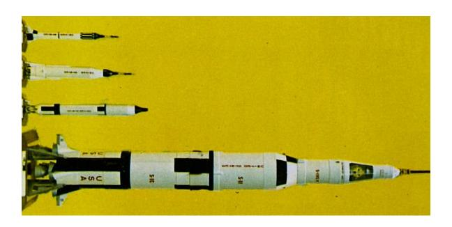
A fully assembled, launch-ready Saturn V stood 363 feet tall and weighed in at roughly 6,000,000 pounds, 90% of which was fuel weight. Depending upon who is telling the story, it contained either 6,000,000 or 9,000,000 parts. There were three disposable launch stages, atop which sat the lunar, service and command modules, which was then capped with a launch escape system that was jettisoned shortly after lift-off.
